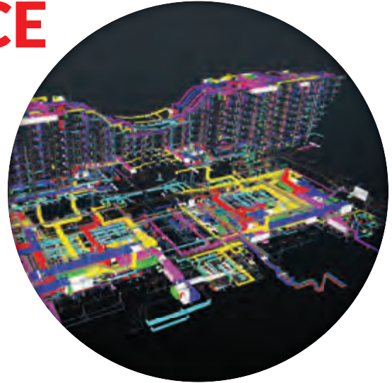
Denver International Airport Westin Hotel, Denver, CO RK leveraged BIM, CAD and field-related applications to prefabricate almost all of the piping—eliminating on-site logistic costs and field welding labor—a big savings of time and money.
